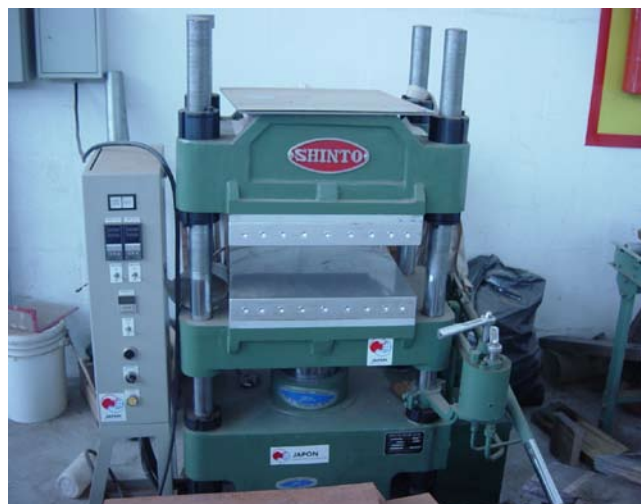
Figura 1. Prensa “SHINTO Compression Moulding Machine”.
